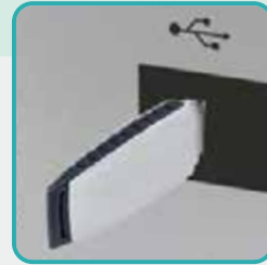
USB port for use with flash drives to record data
