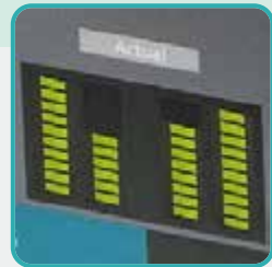
Digital display shows actual suction and irrigation pressures
